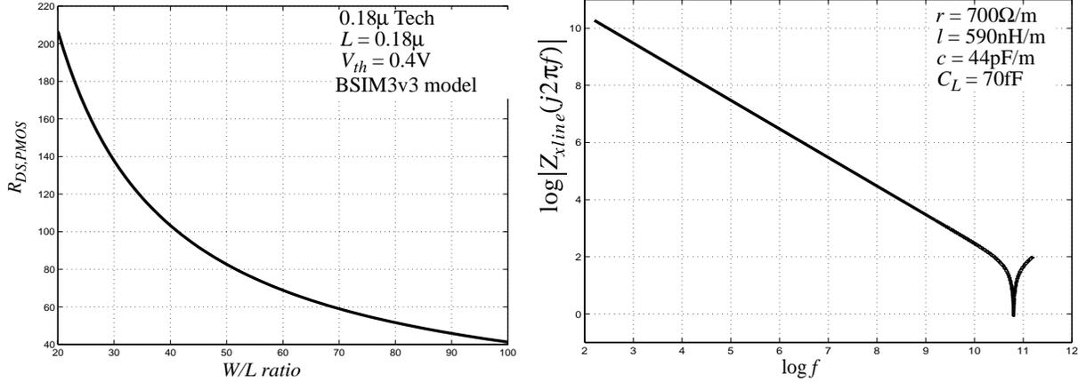
Fig. 11. (a)  $r_{DS, PMOS}$  vs. the gate aspect-ratio (b) the magnitude response of the driving-point impedance of a lossy transmission line
