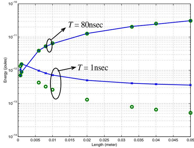
Fig. 16. A comparison between the energy-length variation of the equivalent underdamped RLC- $\pi$  circuit and that of single underdamped RLC circuit of a lossy transmission line. The comparison has been made for two values of cycle time,  $T = 1\text{nsec}$  and  $T = 80\text{nsec}$
