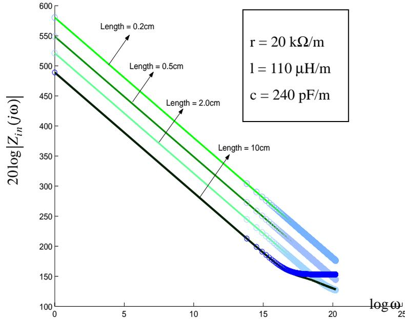
Fig. 8. A comparison between the magnitude response of line's actual driving-point impedance (Eq. (20)) and that of line's approximated rational impedance function (Eq. (26)) for four different line lengths
