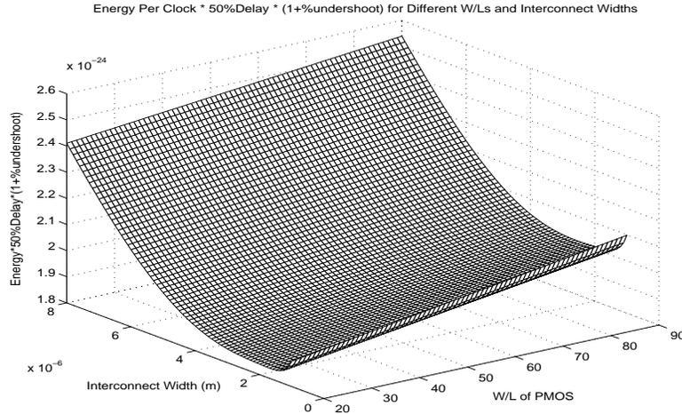
Fig. 15. *EDUP* in terms of W/L and interconnect metal width (RLC- $\pi$ ).
