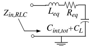
Fig. 8. The circuit realization of Eq. (23)
