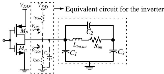
Fig. 12. The equivalent RLC- $\pi$  circuit model of a lossy coupled transmission line driven by a large CMOS inverter
