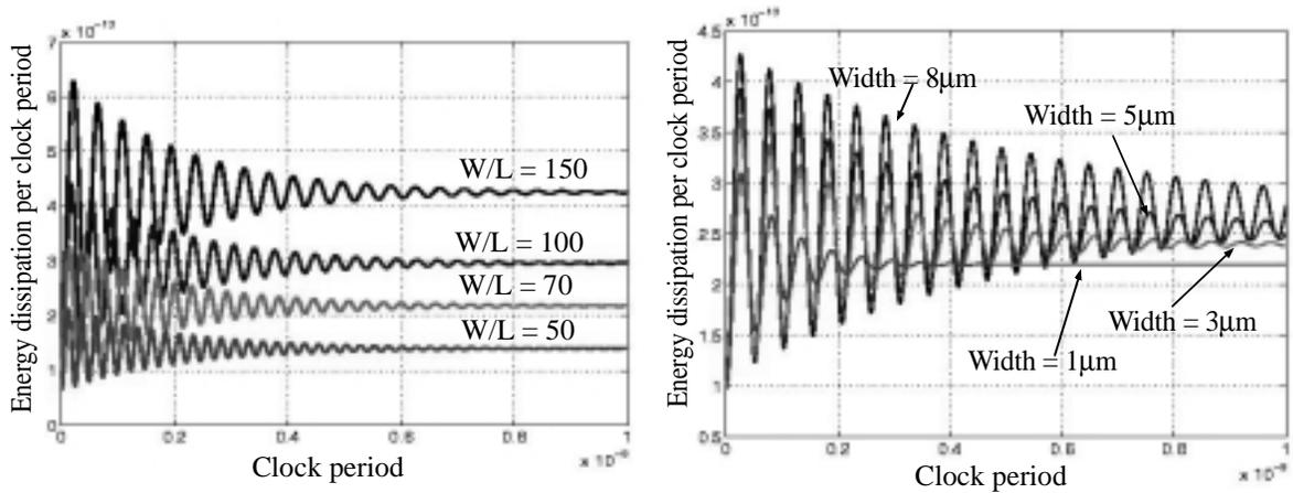
Fig. 13. (a) Energy per clock vs. clock period for six different W/L ratios. (b) Energy per clock vs. clock period for four different interconnect widths (RLC- $\pi$ ).
