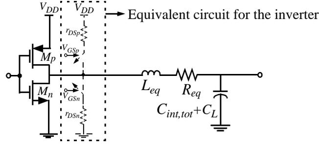
Fig. 18. The equivalent RLC circuit model of a lossy coupled transmission line driven by a small CMOS inverter
