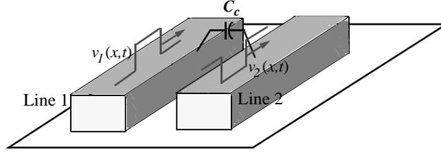
Fig. 6. Two capacitively coupled transmission lines. The traveling voltage waves are 180° out of phase.
