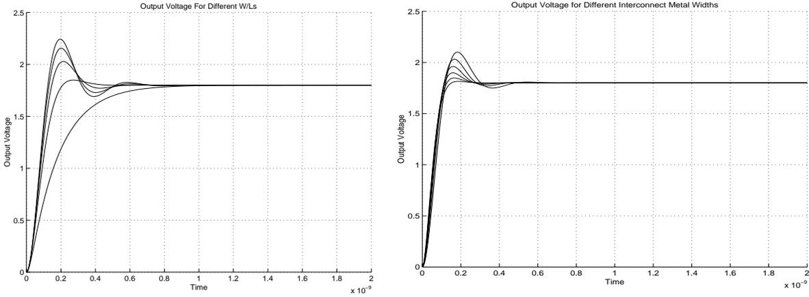
Fig. 20. (a) Voltage waveform for five different W/L ratios (b) Voltage waveform for four different interconnect widths (RLC)
