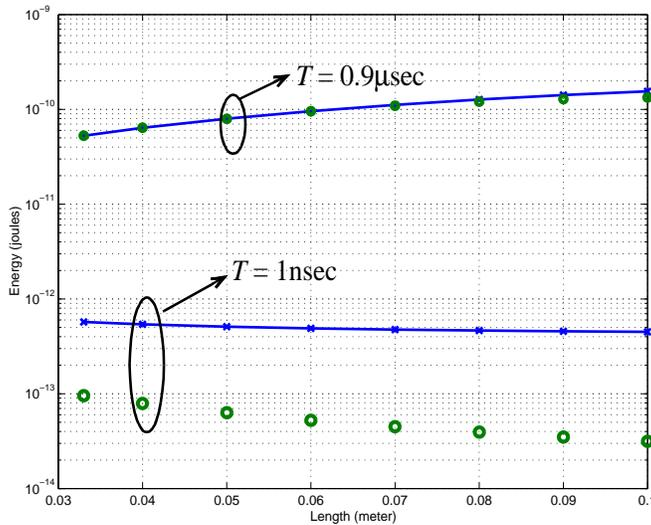
Fig. 17. A comparison between the energy-length variation of the equivalent overdamped RLC- $\pi$  circuit and that of single overdamped RLC circuit modeling a lossy transmission line. The comparison has been made for two values of cycle time,  $T = 1\text{nsec}$  and  $T = 0.9\mu\text{sec}$
