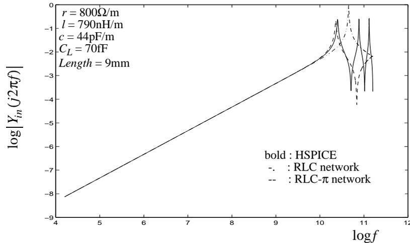
Fig. 10. The magnitude response of the driving-point admittance of an electromagnetically coupled lossy transmission line obtained using HSPICE simulation, and by replacing the line with its equivalent RLC- $\pi$  circuit, and with its equivalent RLC circuit
