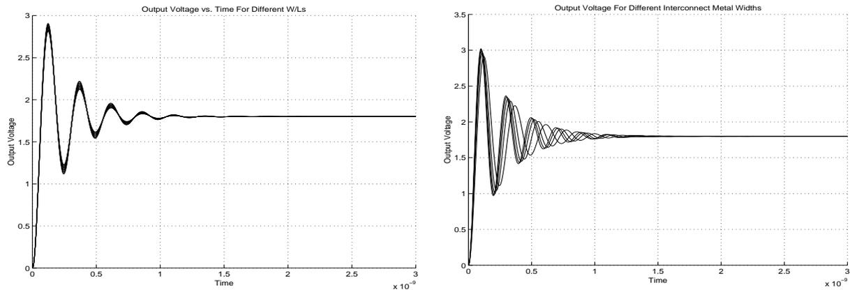
Fig. 14. (a) Voltage waveform for six different W/L ratios (b) Voltage waveform for four different interconnect widths (RLC- $\pi$ )
