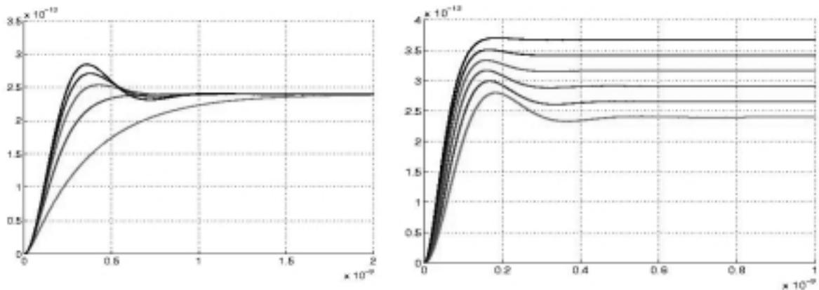
Fig. 19. (a) Energy per clock vs. clock period for five different W/L ratios (b) Energy per clock vs. clock period for six different interconnect widths (RLC)
