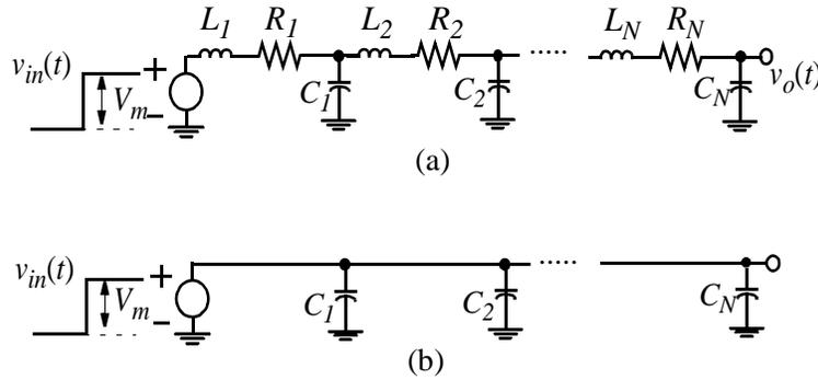
Fig. 4. A ladder of cascaded RLC circuits. (a) the circuit schematic. (b) the equivalent circuit for the energy analysis
