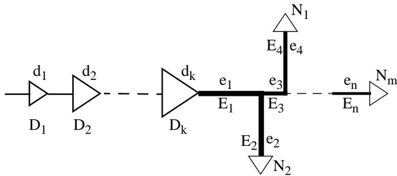
Figure 6 A k-stage cascaded driver driving an tree with m sinks
