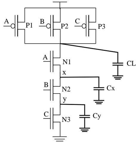
Figure 5 Effect of signal reordering on power dissipation
