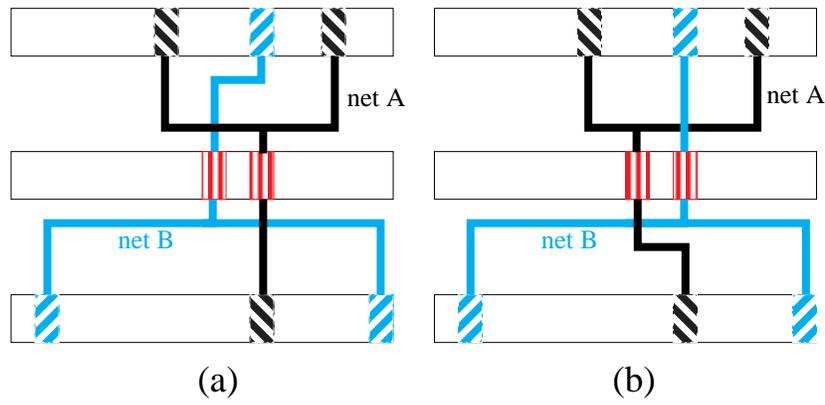
Figure 3 Effect of switching activity on Feedthrough assignment
