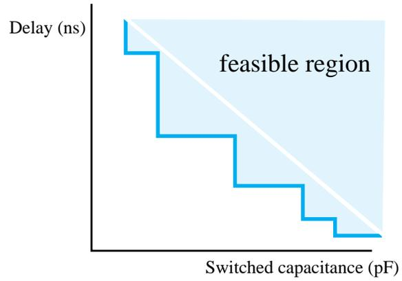
Figure 4 A power-delay tradeoff curve
