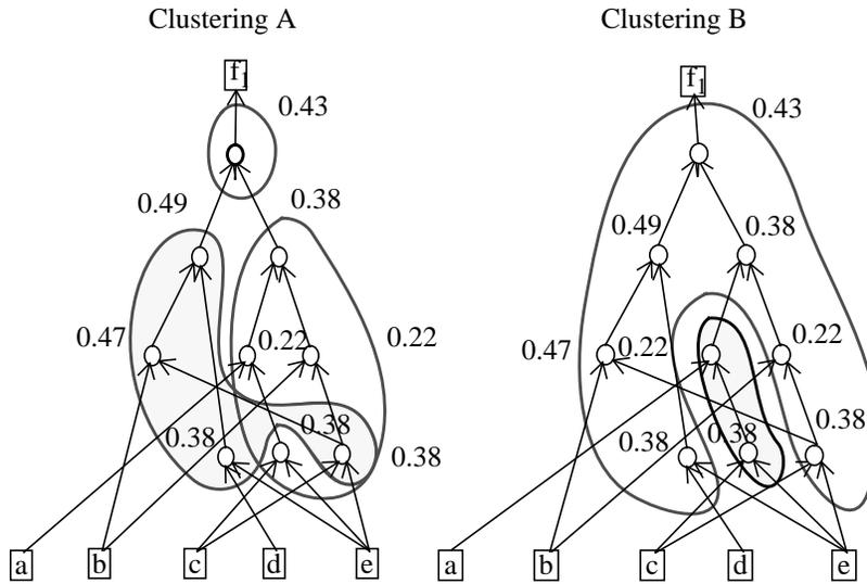
Figure 2 Clustering solutions with equal logic depth but different power.
