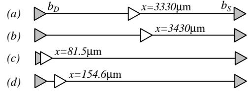
Fig. 5. Location of an inserted buffer in a 6660  $\mu\text{m}$  line (0.18  $\mu\text{m}$  technology): (a) standard technique (b) temperature-aware technique with only variable  $r$  (c) temperature-aware technique with only variable  $R_d$  (d) temperature-aware technique with both variable  $R_d$  and  $r$ .
