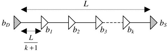
Fig. 3. Structure of standard buffer insertion in a uniform line with equal segmentation.
