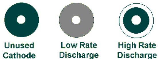
**Figure 4 The "cathode freeze over" phenomenon of the Li/SOCl<sub>2</sub> battery**
