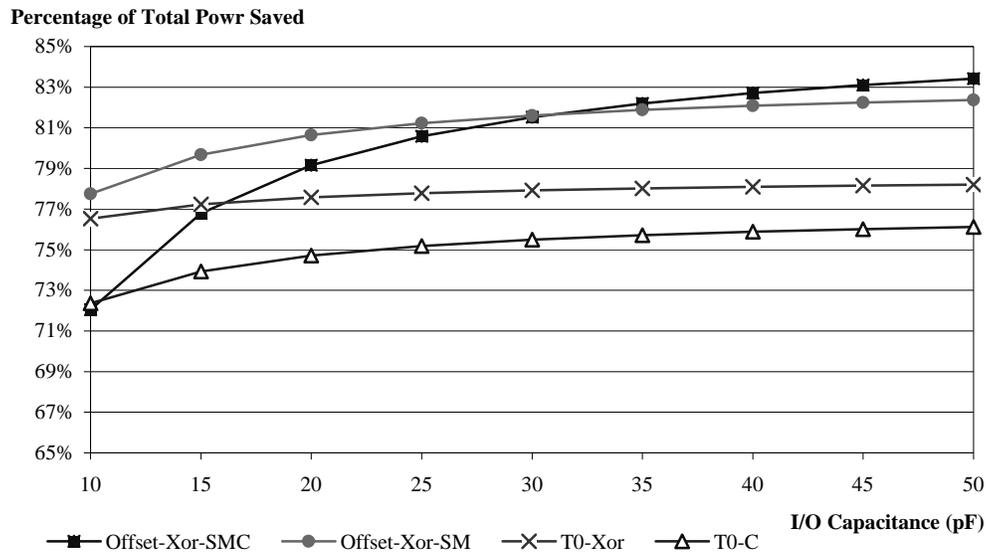
Figure 6- Comparison of total power savings for several encoding techniques.
