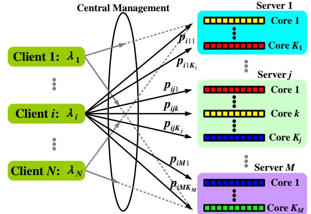
**Figure 1:** Architecture of the resource allocation problem in the cloud computing system.
