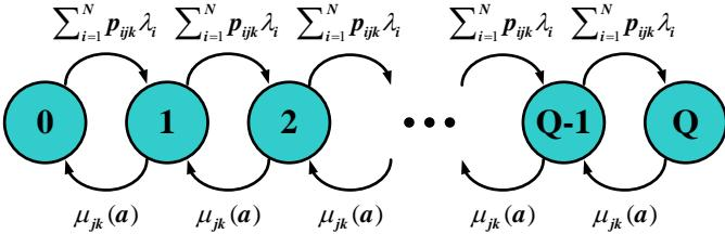
Figure 2: CTMDP model of the SQ in each core.
