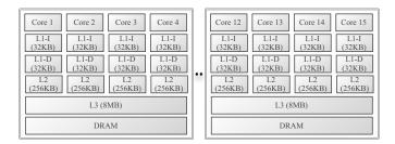
Fig. 9. Topology of 16 cores (four 4-core processors) in Sniper simulation.
