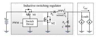
Fig. 2. Circuit schematics of a inductive (synchronous) switching VR.
