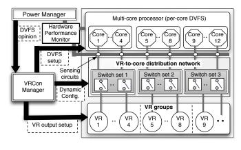
Fig. 4. Diagram of the proposed multicore platform.
