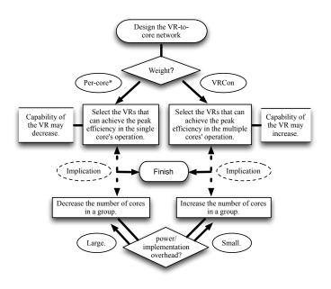
Fig. 6. Design flows to determine the VRs and the number of network switches in the proposed platform. Per-core\* in the figure means that a designer puts more weight on the energy saving of the VR by setting it to achieve the best efficiency in the normal operation condition of each core.
