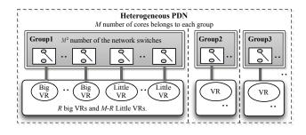
Fig. 7. A part of the proposed platform with the heterogeneous VRs: each group has the R big VRs and M-R little VRs
