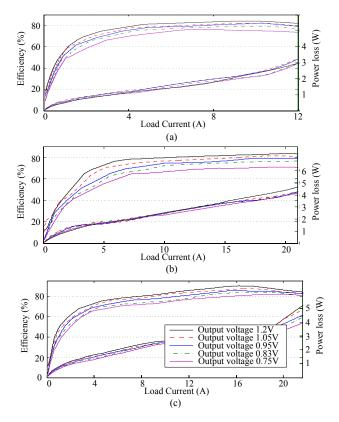
Fig. 11. Efficiency and Power loss vs. Load current for LTC3816 with (a) Si4840DY, (b) Si4838DY and (c) Si4442DY.
