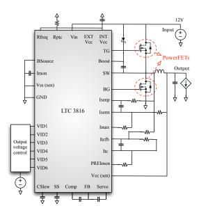
Fig. 10. VR schematic used in the spice simulation.
