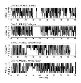
Fig. 8. A part of the per-core DVFS results of *Barnes* and *Streamcluster* from the Sniper simulation with 4-core setup.
