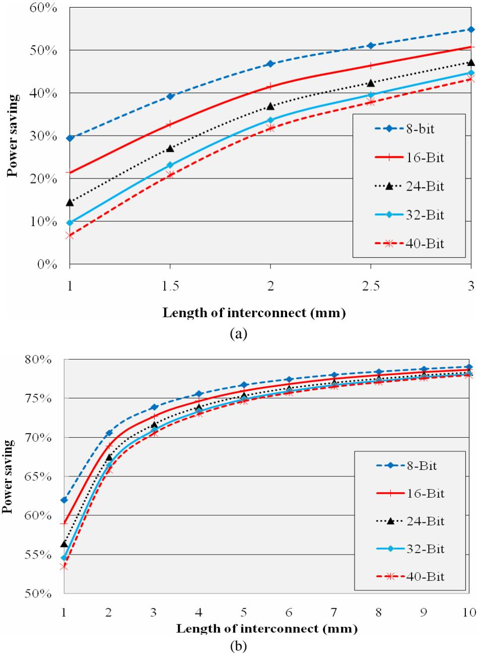
**Figure 7.** The power savings achieved through coding as a function of the length for different bus widths. (a) On-chip buses (b) off-chip buses.
