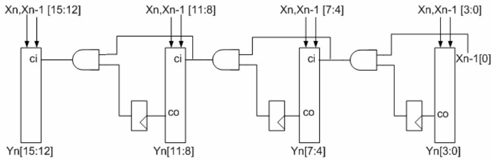
**Figure 5.** Modified version of DX architecture (called registered DX.)
