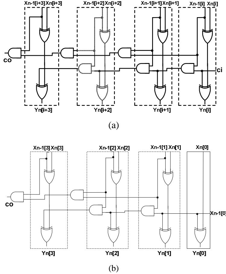
**Figure 6.** (a) Basic block (other than the first block) of registered DX architecture for  $M = 4$ . (b) First block of registered DX architecture for  $M = 4$ .
