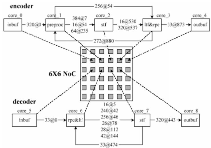
**Fig. 8 Partition, communication trace and core mapping of a GSM voice CODEC [25]**
