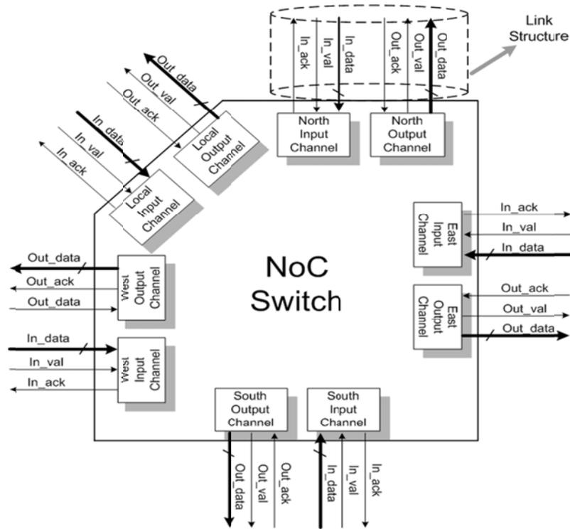
**Fig. 1 Proposed switch interface and architecture.**
