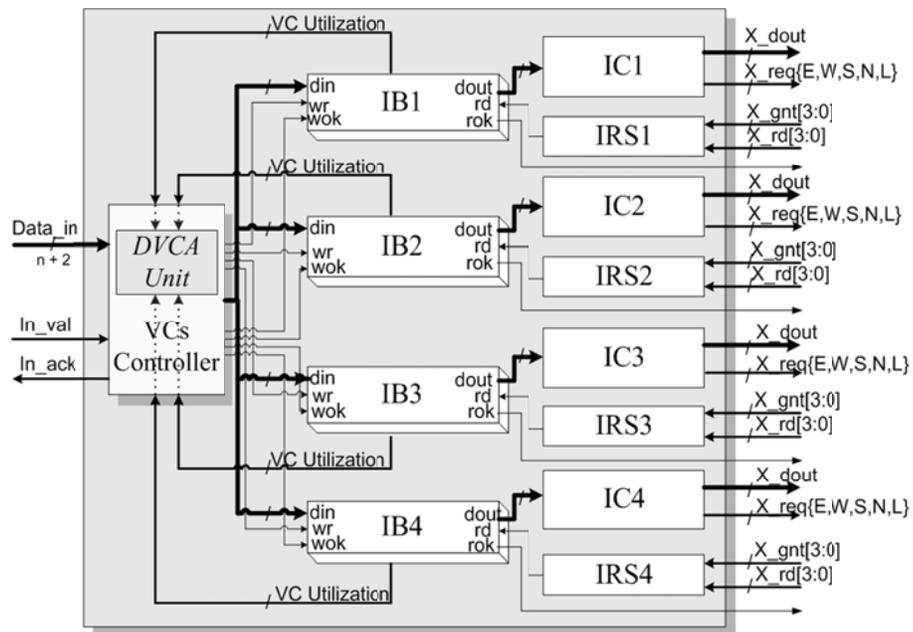
**Fig. 2 Input channel architecture.**
