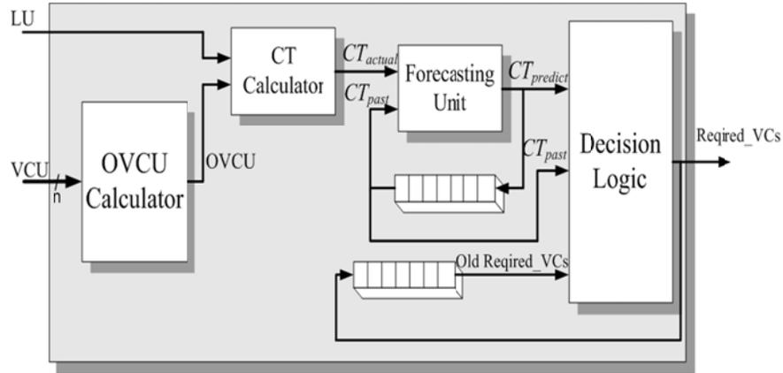
**Fig. 5** The hardware diagram of the forecasting-based DVCA policy.
