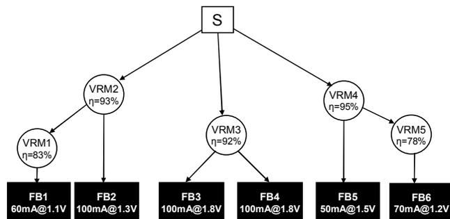
Figure 10 : VRM tree topology in testbench 1.
