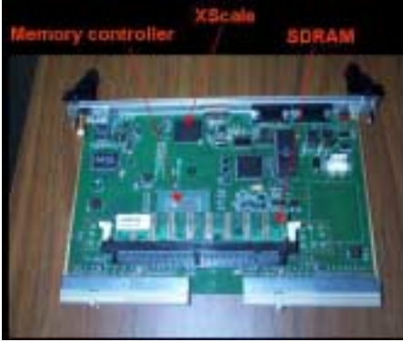
Fig. 6. Main board with the CPU, memory, and memory controller
