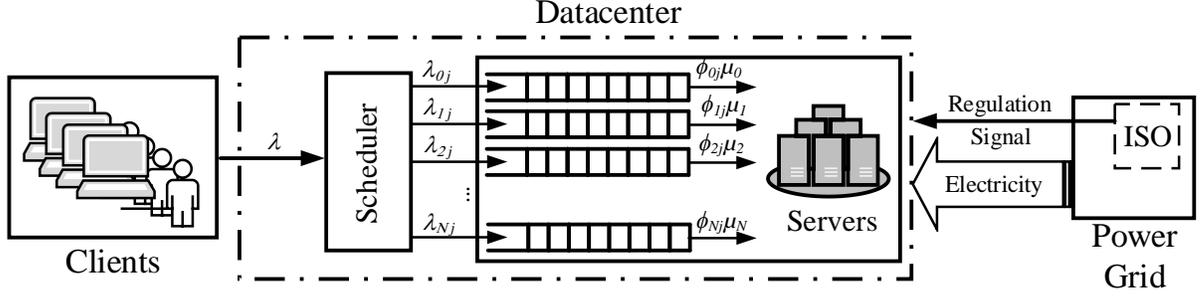
Fig. 1 The overview of the data center system.
