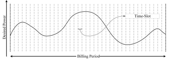
Fig. 2 Regulation signal over a billing period.
