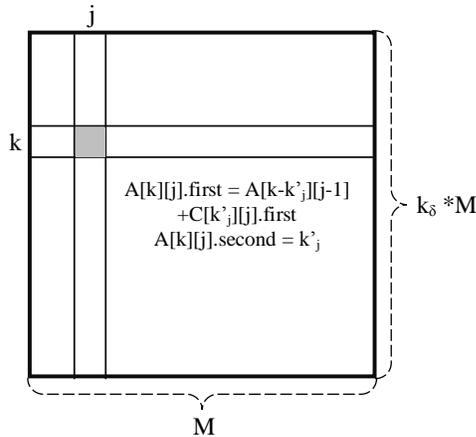
Fig. 3 Dynamic programming matrix (Matrix  $A$ ) constructed to solve the problem over the billing period.
