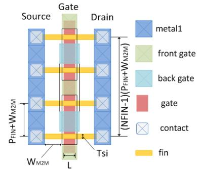
**Figure 6: Layout of an independent gate FinFET device with four fins.**
