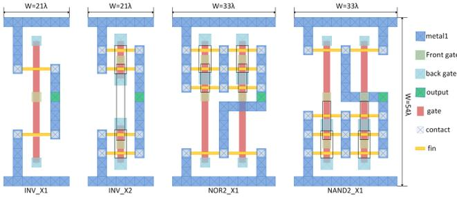
**Figure 7: 7nm FinFET independent-gate layout of inverters, 2-input NAND gates and 2-input NOR gates**
