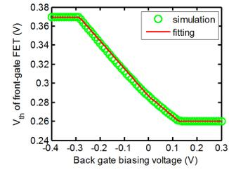
Figure 2:  $V_{th}$  of the front-gate-controlled N-type FET vs. back-gate voltage.
