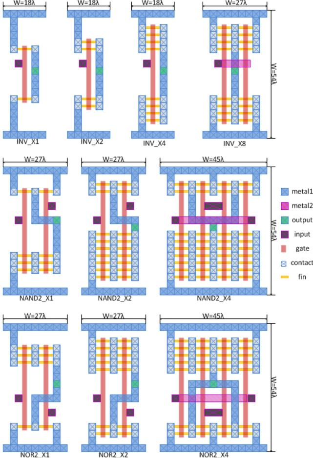
**Figure 5: 7nm FinFET shorted-gate layout of inverters, 2-input NAND gates and 2-input NOR gates with different sizes**
