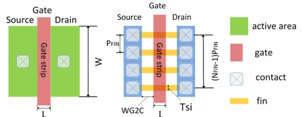
**Figure 4: Layout of (a) a general CMOS device and (b) a shorted-gate FinFET device with four fins.**
