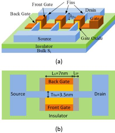
Figure 1: (a) Perspective view and (b) top view of the 7nm FinFET device.
