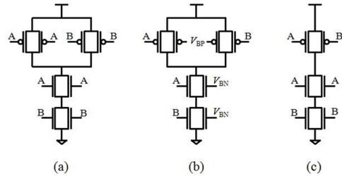
Figure 3: Different FinFET-based NAND gate designs.
