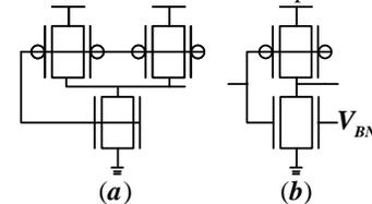
Figure 2. Different FinFET inverters in different modes.
