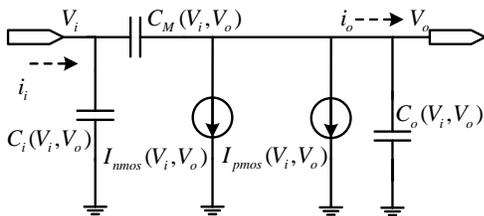
Figure 3. Equivalent CSM for a CMOS inverter [14].
