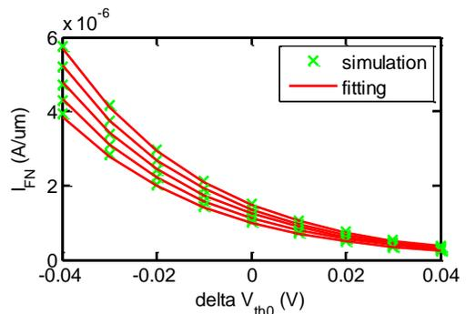
Figure 6. Curve fitting of N-type FET driving current under different corners of process variation.
