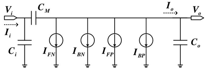
Figure 5. Equivalent CSM for a FinFET inverter.
