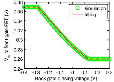
Figure 1.  $V_{th}$  of front-gate-controlled N-type FET v.s. back-gate voltage.
