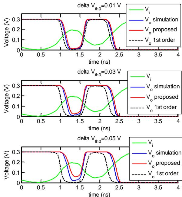
Figure 7. Output waveforms for different CSM variation handling techniques under a noise input at different threshold voltage variation levels.
