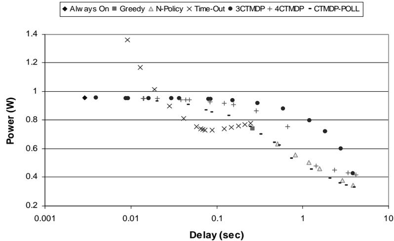
Power-delay trade-off curves for Uniform transition time distribution for the hard disk and a combination of Exponential and Pareto distributions for the request inter-arrival times
