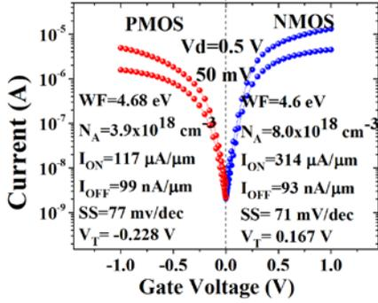
Fig. 2  $I_{DS}$ - $V_{GS}$  characteristics of JL-GAA NMOS/PMOS. The performance parameters are measured at  $V_{DD}=0.5$  V. Current values are normalized to effective channel width  $(W_{si}+H_{si}) \times 2$ .
