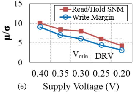
Fig. 6 8T SRAM design simulation at different supply voltage. (a). access latency; (b). access energy; (c). noise margin; (d). leakage power; (e). Hspice monte carlo variation simulation. The sample number is 1000.
