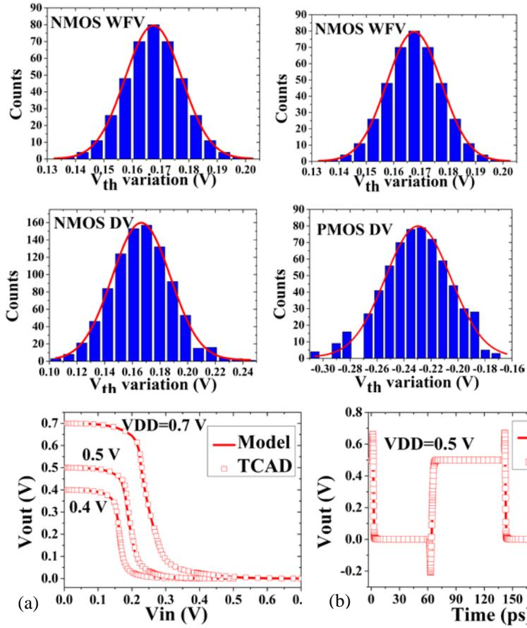
Fig. 3 NMOS/PMOS threshold voltage ( $V_{th}$ ) variation due to work function variation (WFV) and doping variation (DV). The standard deviations of WFV and DV are assumed to be  $\sim 20$  meV and 20%, respectively.
